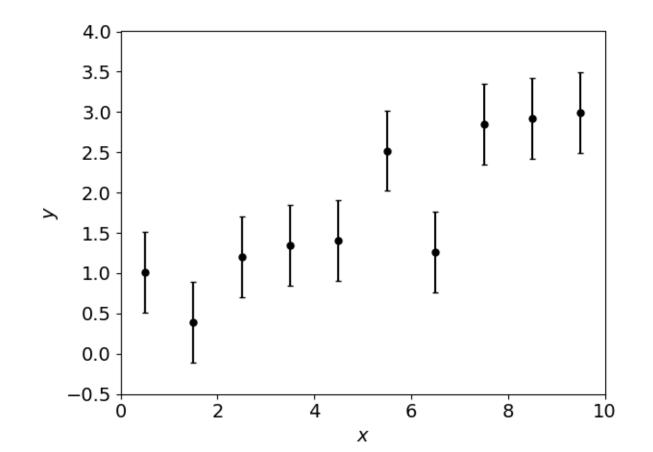
• Could these points be fit by a constant y = b? Minimizing  $\chi^2$ , we find  $\chi^2_{min} = 31.6$  for b = 1.79
