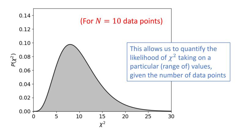
• Sampling many realizations of N data points from a particular model, using Gaussian statistics, the  $\chi^2$  statistic has a **probability distribution**
