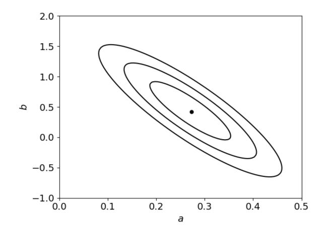
• What about errors in individual parameters? For each value of parameter a, find the minimum  $\chi^2$  varying parameter b:
