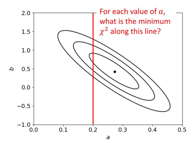
• What about errors in individual parameters? For each value of parameter a, find the minimum  $\chi^2$  varying parameter b:
