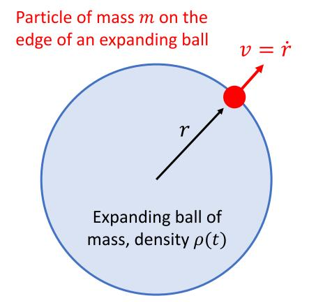
Conservation of energy for the particle:  $\frac{1}{2}m\dot{r}^2 - \frac{GM(< r)m}{r} = E$ Writing  $M(< r) = \frac{4}{3}\pi r^3 \rho(t)$  and using comoving coordinates  $r(t) = a(t) r_0$ , this equation becomes,  $\left(\frac{\dot{a}}{a}\right)^2 = \frac{8\pi G \ \rho(t)}{3} - \frac{c}{a^2}$
