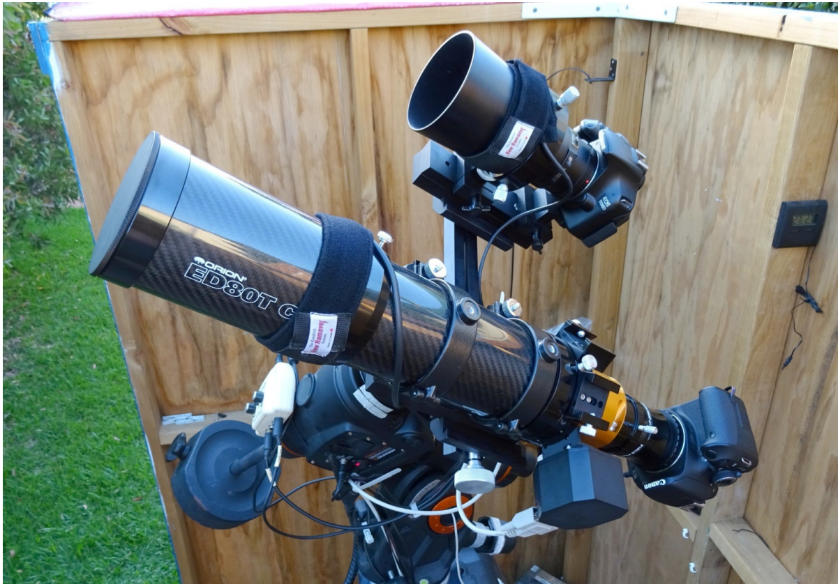
Mark Blackford's dual DSLR photometry system. Canon EOS 1100D with 200mm f2.8 lens (6.5° x 4.3°) Canon EOS 600D with 80mm f6 telescope (2.7° x 1.8°)
