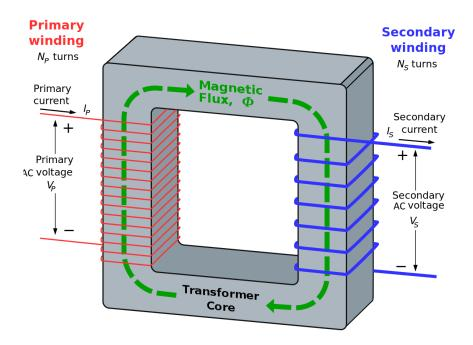
Faraday's law says that an electric current is set up if the magnetic field through a circuit is changed
