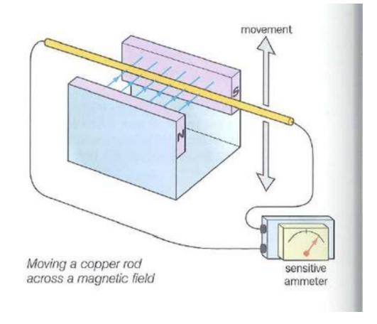
• A voltage is induced between the ends of the wire which is equal to the rate of cutting of magnetic flux,  $V = -\frac{\partial \Phi}{\partial t}$
