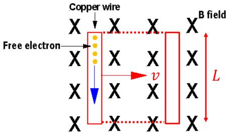
Copper Wire Moving To The Right In A Magnetic Field
